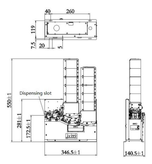
Module dimension: 346.5mm(L)×140.5mm(W)×550mm(H)
