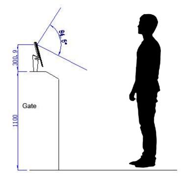
The camera elevation angle can be adjusted to  $0^{\circ}$ ,  $5^{\circ}$ ,  $10^{\circ}$ ,  $15^{\circ}$ , and  $20^{\circ}$ . The bracket fixing screws can be adjusted according to the on-site conditions.
